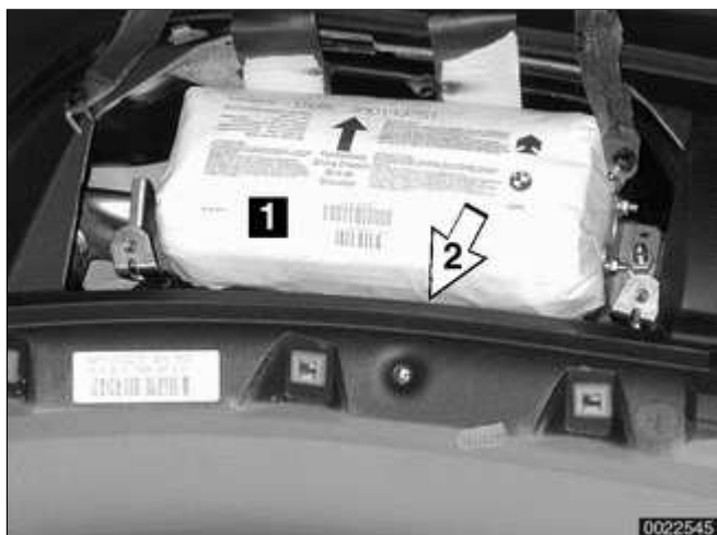
◀ Fig. 41 Right side dashboard 1 - Passenger airbag 2 - Passenger airbag connector
