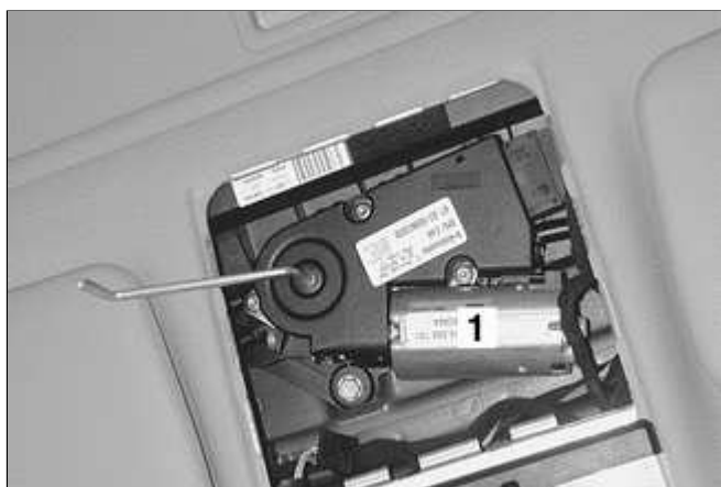
◀ Fig. 43 In headliner 1 - Sunroof motor
