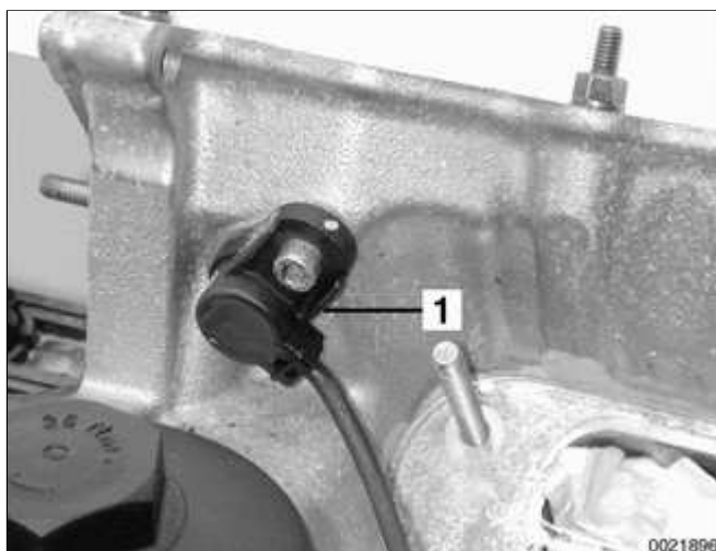
◀ Fig. 28 Cylinder head, left front 1 - Intake camshaft position sensor
