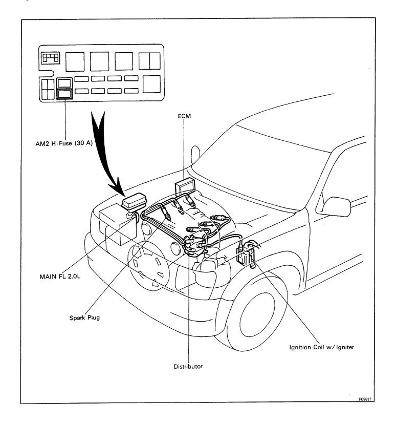
The ECM monitors the engine condition by signals from each sensor, calculates the ignition timing and sends an ignition signal to the igniter. High voltage from the ignition is distributed to each spark plug in the appropriate order to generate a spark between the electrodes, which ignites the air–fuel mixture.
