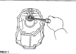
2. (4WD) IF NECESSARY, REPLACE TRANSFER ADAPTOR OIL SEAL
