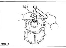
(b) Using SST and a hammer, drive in a new oil seal. SST 09325-12010
