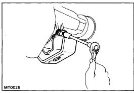
(d) Remove the engine rear mounting from the transmission.
