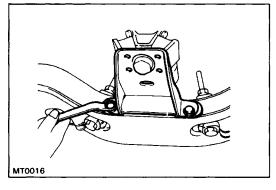
(c) Remove the four bolts from the support member and remove the mounting bracket.
