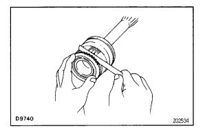
(c) Using a feeler gauge, measure the clearance between the synchronizer ring back and the gear spline end. Minimum clearance:
