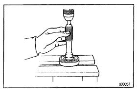
(b) Using a press, remove the bearing.
