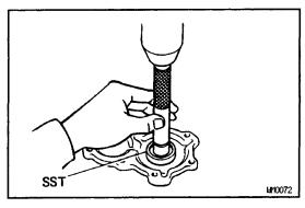
(b) Using SST and a press, install a new oil seal. SST 09608–20012 (09608–03020, 09608–00080) **Drive in depth:**
