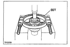
(b) Using SST and a press, remove the bearing. SST 09950–00020
