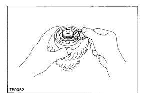
(f) Select a snap ring that will allow minimum axial play and install it on the shaft.
