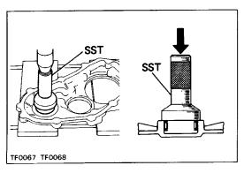
(b) Using SST and a press, press in a new bearing. SST 09310–3 5010
