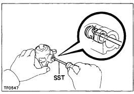
(c) Using SST, pull out the seat. SST 09921–00010
