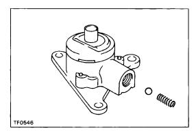
(b) Using a magnetic finger, remove the spring and ball.
