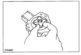
(c) Install the drive rotor.
