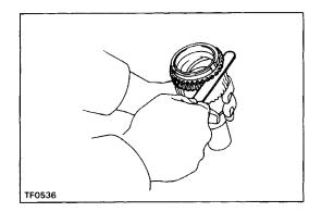
(b) Measure the clearance between the synchronizer ring back and the input shaft spline end.
