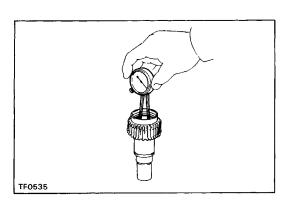
(b) Using a dial indicator, measure the inside diameter of the input shaft bushing.
