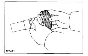
(b) Remove the sun gear from the input shaft.
